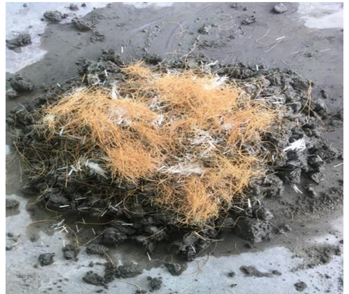
Fig. 4 Mixing of Hybrid Fibres
